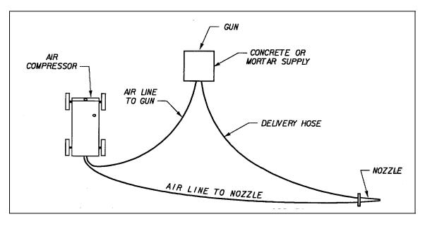
Figure 4-6. Typical plant layout for wet-mix pneumatic-feed equipment
