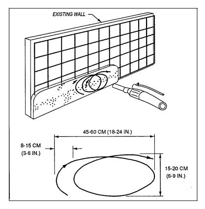
Figure 6-2. Shotcrete nozzle motion (after Ryan 1973)
