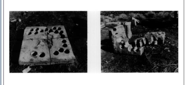
Figure 5-3. Cored and quartered test panels
